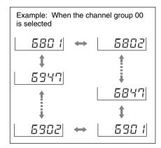
**6** When the desired channel number appears, leave the tuner for about 10 seconds until the selected channel number stops flashing and the selection is stored in memory.
